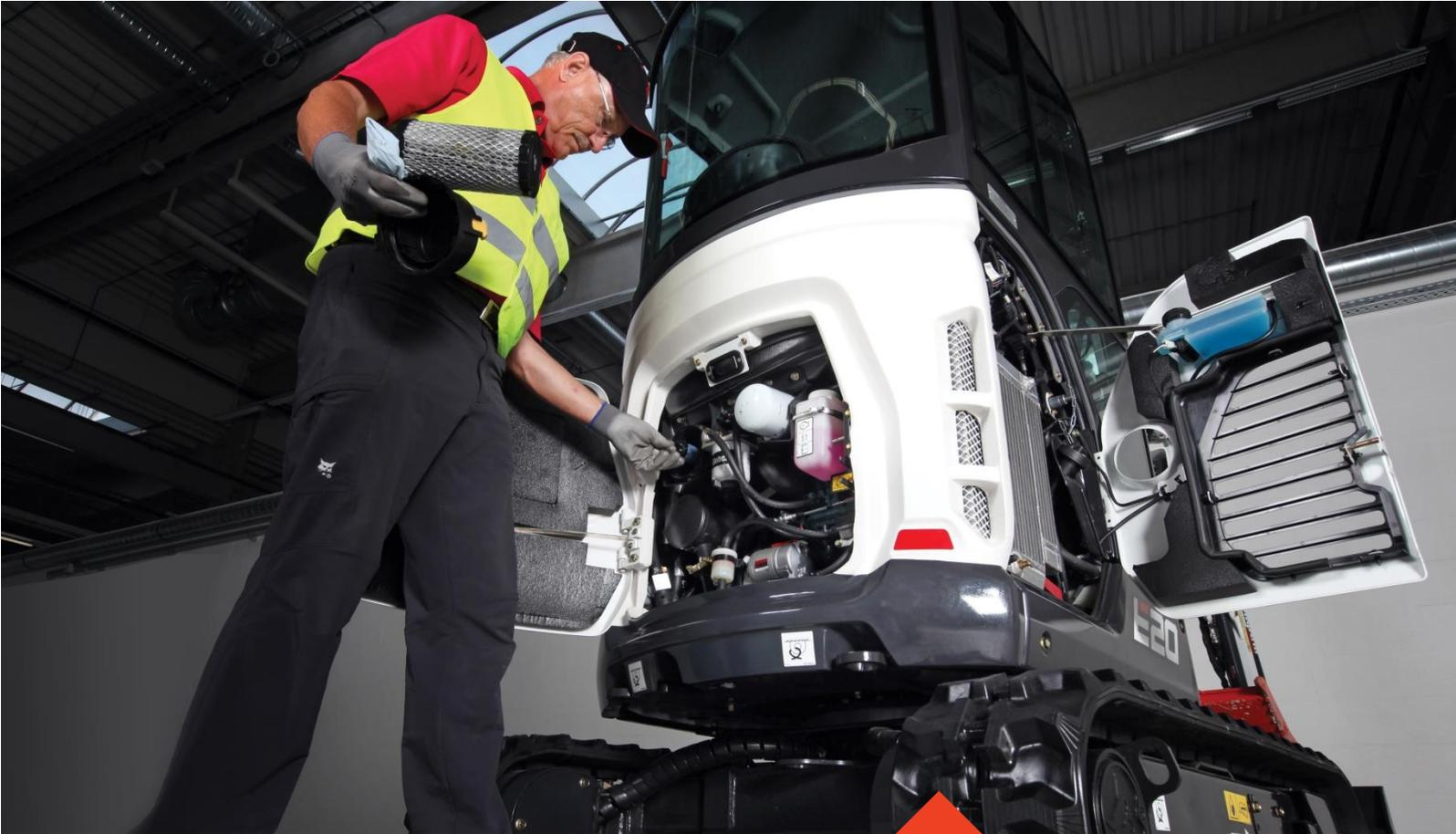
Side-by-side coolers for easy cleaning. Diagnostics are easy thanks to display error codes on control panel and service tool connection. The E20 tailgate provides great access to all daily maintenance components and service points.
